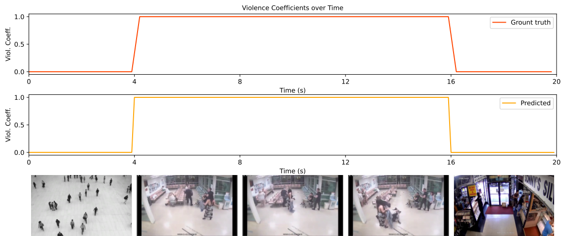
Figure 3.20: Results of my standalone system using FT model on a video compiled from 3 random videos of Smart-City CCTV Violence Detection Dataset, one violent and two non-violent videos concatenated in such a way that the violent video is placed in between two non-violent videos. Row 1: Ground truth of violence coefficients over time. Row 2: Predicted violence coefficients on 4-second video segments. Row 3: Keyframes extracted from the video (original illustration by Viktor Huszár).
